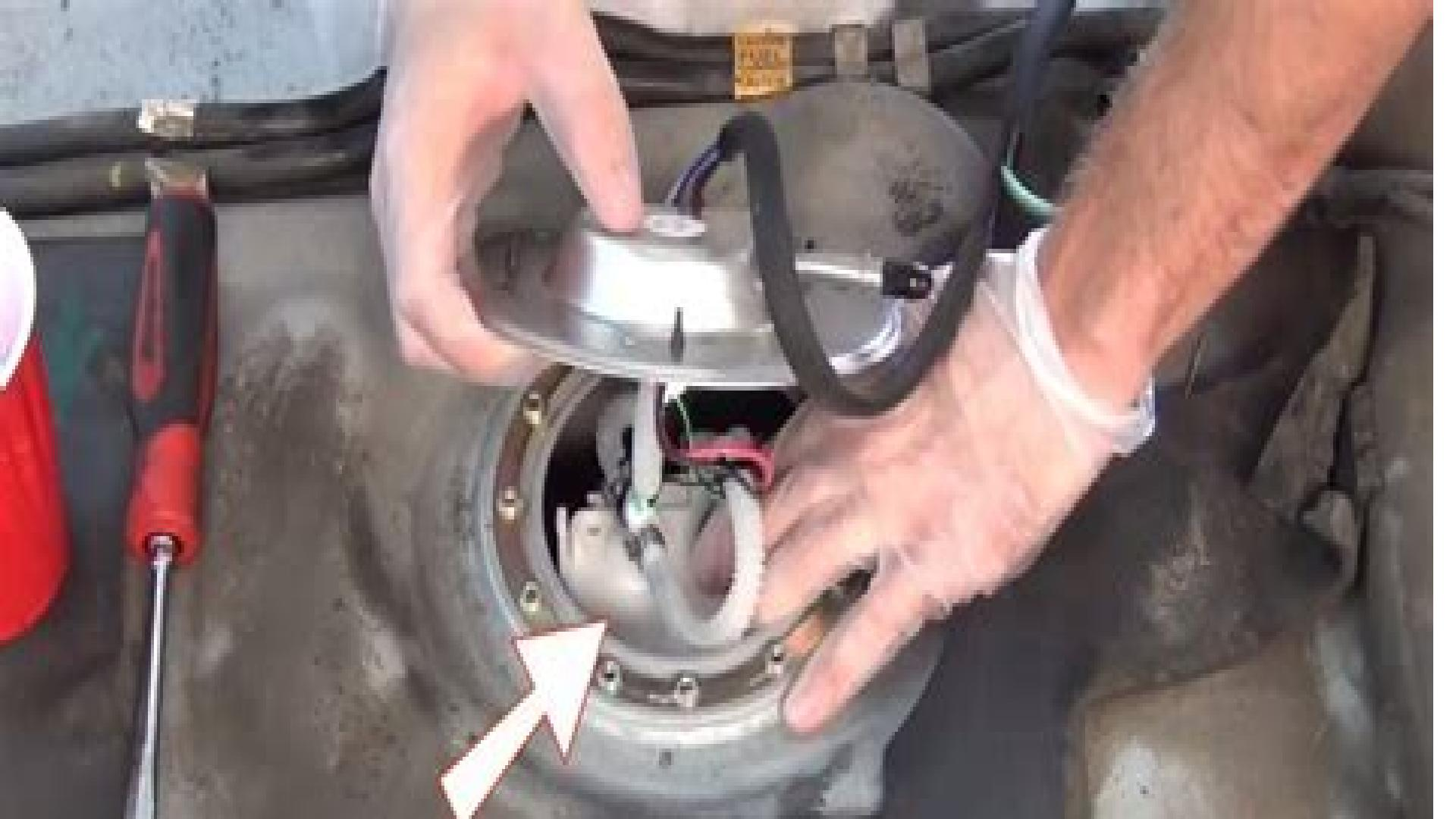
New Fuel Pump Installed
