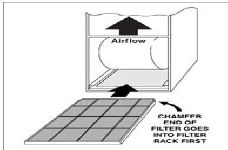
The furnace filter may be secured with filter retaining brackets for right side return on smaller furnaces. To replace filters on these furnaces, remove the blower access door, push back to flex the filter and clear the filter retaining bracket at the front of the unit. Gently pull the filter out.
