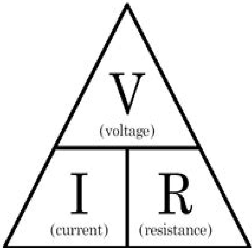
A triangle with vertices labeled **V** at the top, **I** at the bottom left, and **R** at the bottom right. The top edge is labeled **V =** and the bottom edge is labeled **I \* R**.
