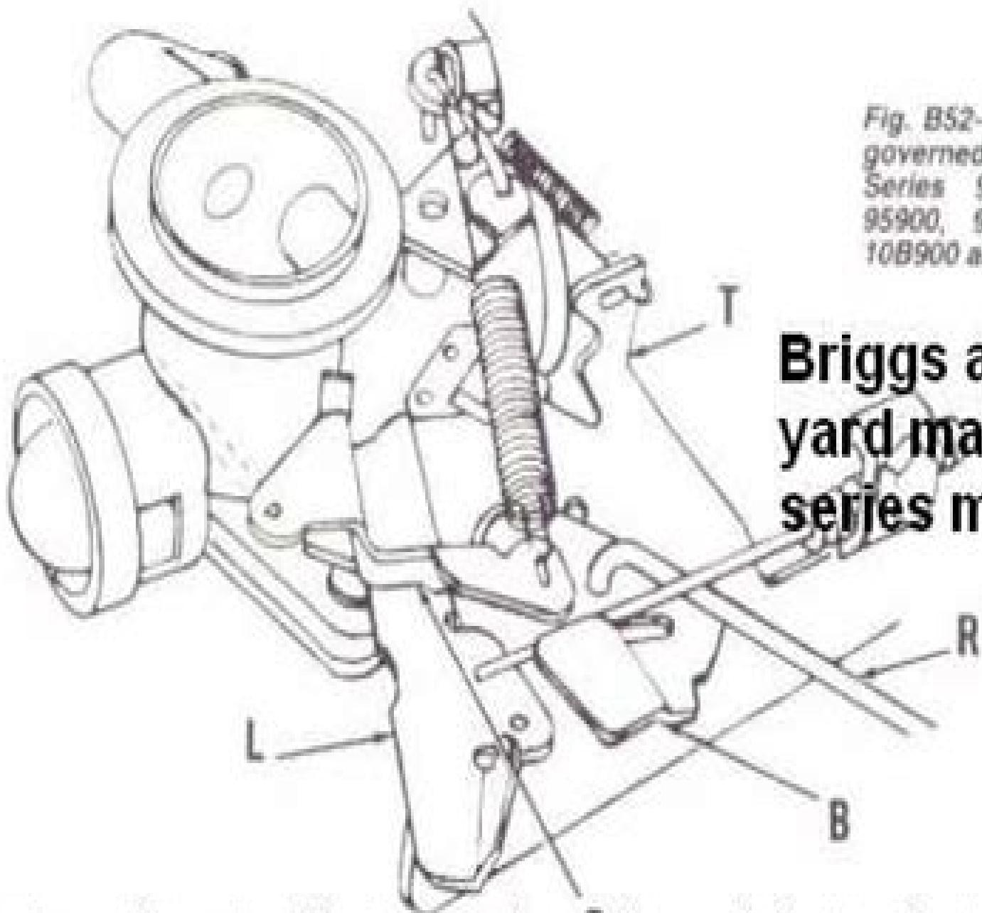
Fig. B52—Refer to text to adjust governed top no-load speed on Series 9B900, 9C900, 9390, 95900, 96900, 98900, 10A900, 10B900 and 10C900.
