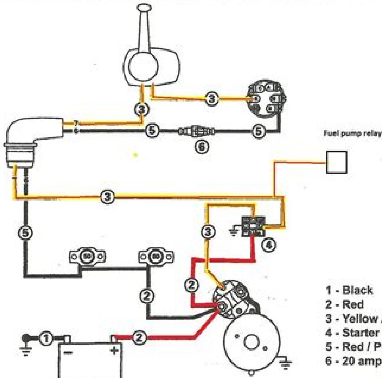
Fig. 160 Starting system wiring schematic—1996-98 3.0L, 4.3L and 5.7L engines (carburetor)
