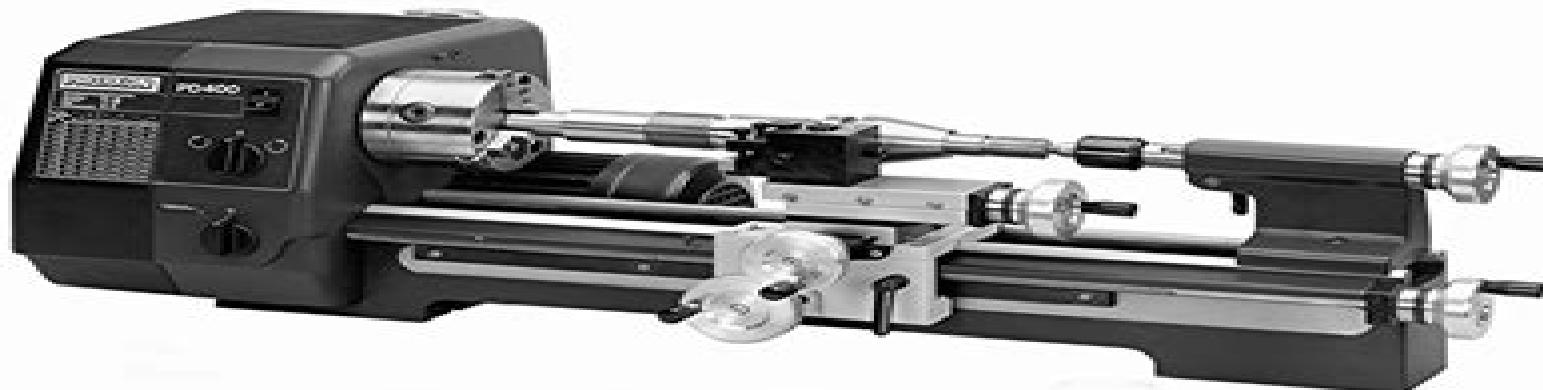
*For someone with limited space a variety of small lathes are available. This photograph shows a Proxxon which is an ideal example. It is quite capable of doing very good work and at the same time is small enough to be put away in a cupboard or even a deep drawer when not in use. It has an electronic speed control system and it is possible to purchase a whole range of accessories in order to increase the versatility of the machine.*
