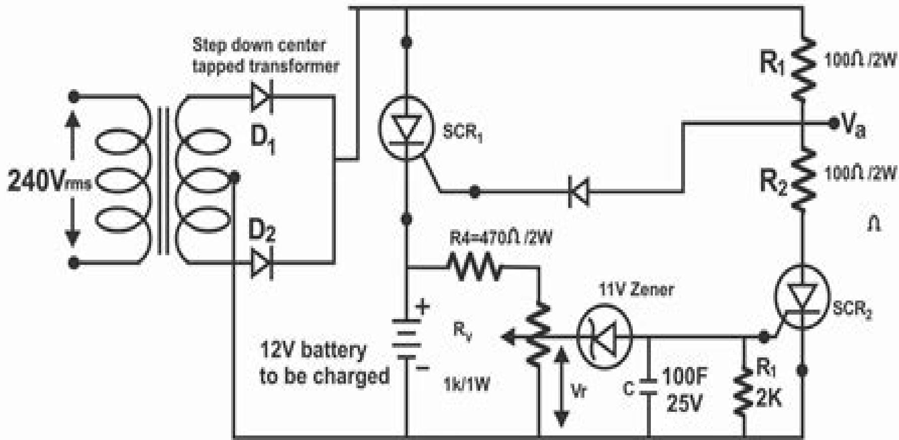
Fig 6.30 A battery charger using two SCRs
