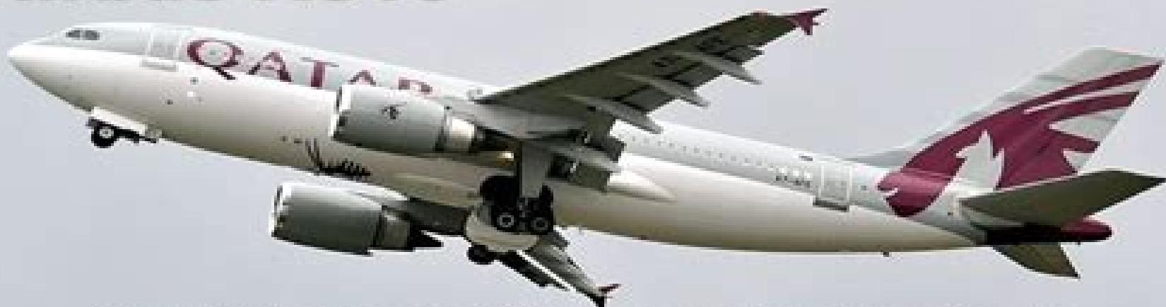
Shorter fuselage than the A300, and only two doors along the fuselage
