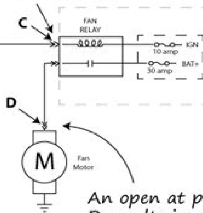
An open at point D results in no fan motor operation.
