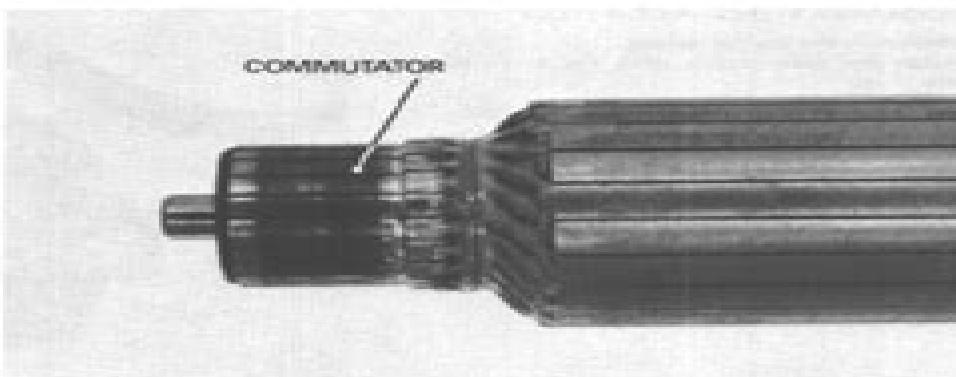
Check for continuity between pairs of commutator bars, and also between commutator bars and armature shaft.
