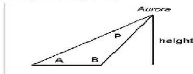
**Question 1** - Suppose that two observers were located 30 kilometers apart. Observer A measured an angle of 53 degrees and Observer B measured an angle of 114 degrees. By making a scaled drawing of this triangle, what was the height of the auroral feature they were studying?
