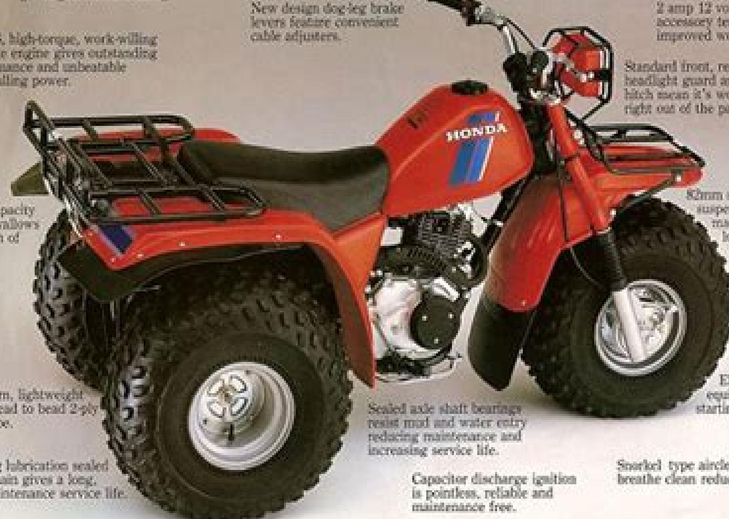
Sealed axle shaft bearings resist mud and water entry reducing maintenance and increasing service life.
