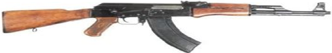
Kalashnikov AK (the original AK-47 with combination stamped / milled receiver)
