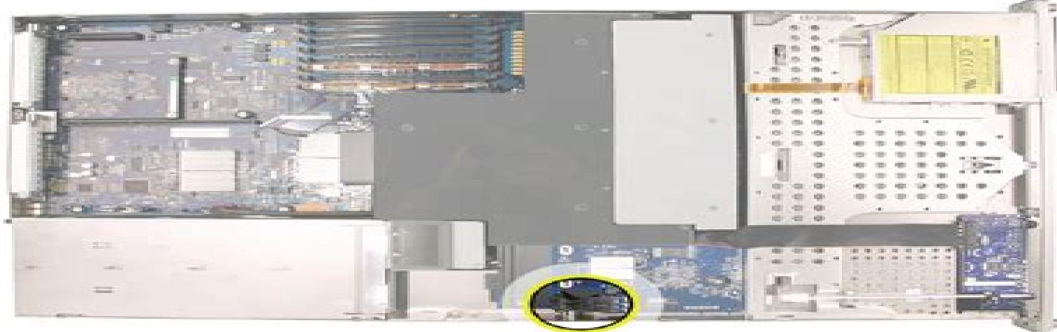
2. Disconnect the power distribution board cable from its connector on the drive interconnect backplane.
