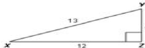
$$\text{Sine}(x) = \text{Perpendicular}/\text{Hypotenuse} = 5/13$$
