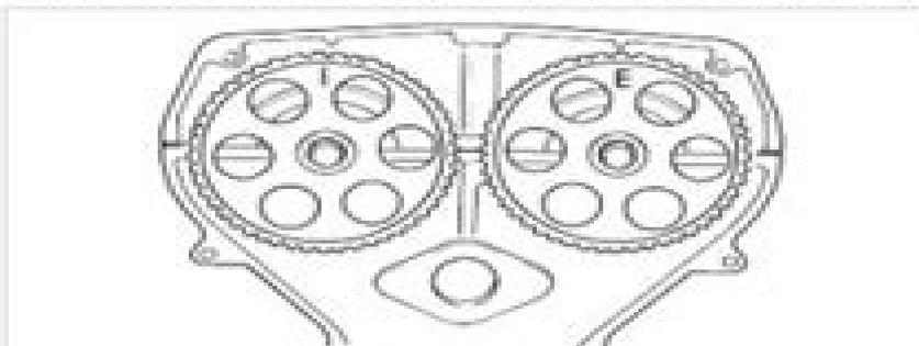
3. Install the camshaft after lubricating the journal of camshaft with engine oil.
