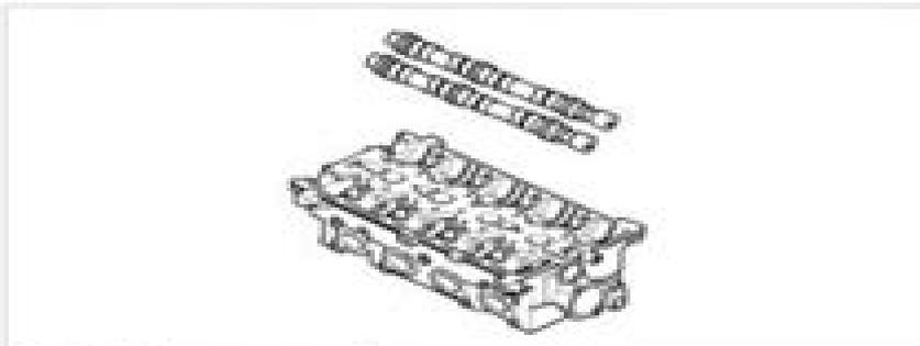
4. Install the cam carrier assembly.
