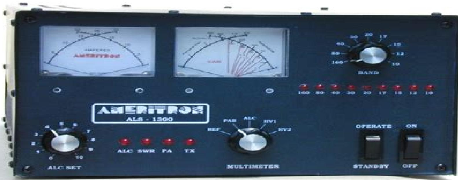
The Ameritron ALS-1300 is 160 through 15-meter amateur radio band 1200-watt output solid-state amplifier. It uses eight 50-volt conservatively rated linear RF MOSFETS. 50-volt linear FET's designed for transmitting service produce an exceptionally clean signal compared to other solid-state amplifiers. Fan speed is regulated by temperature sensors; assuring conservative cooling with minimum noise.
