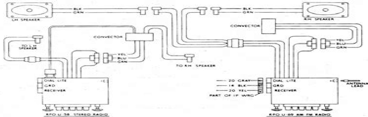
Wiring diagram for 1973 models - mono and stereo radios
