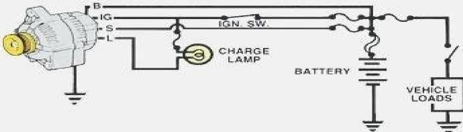
Four wires connect the alternator to the rest of the charging system.
