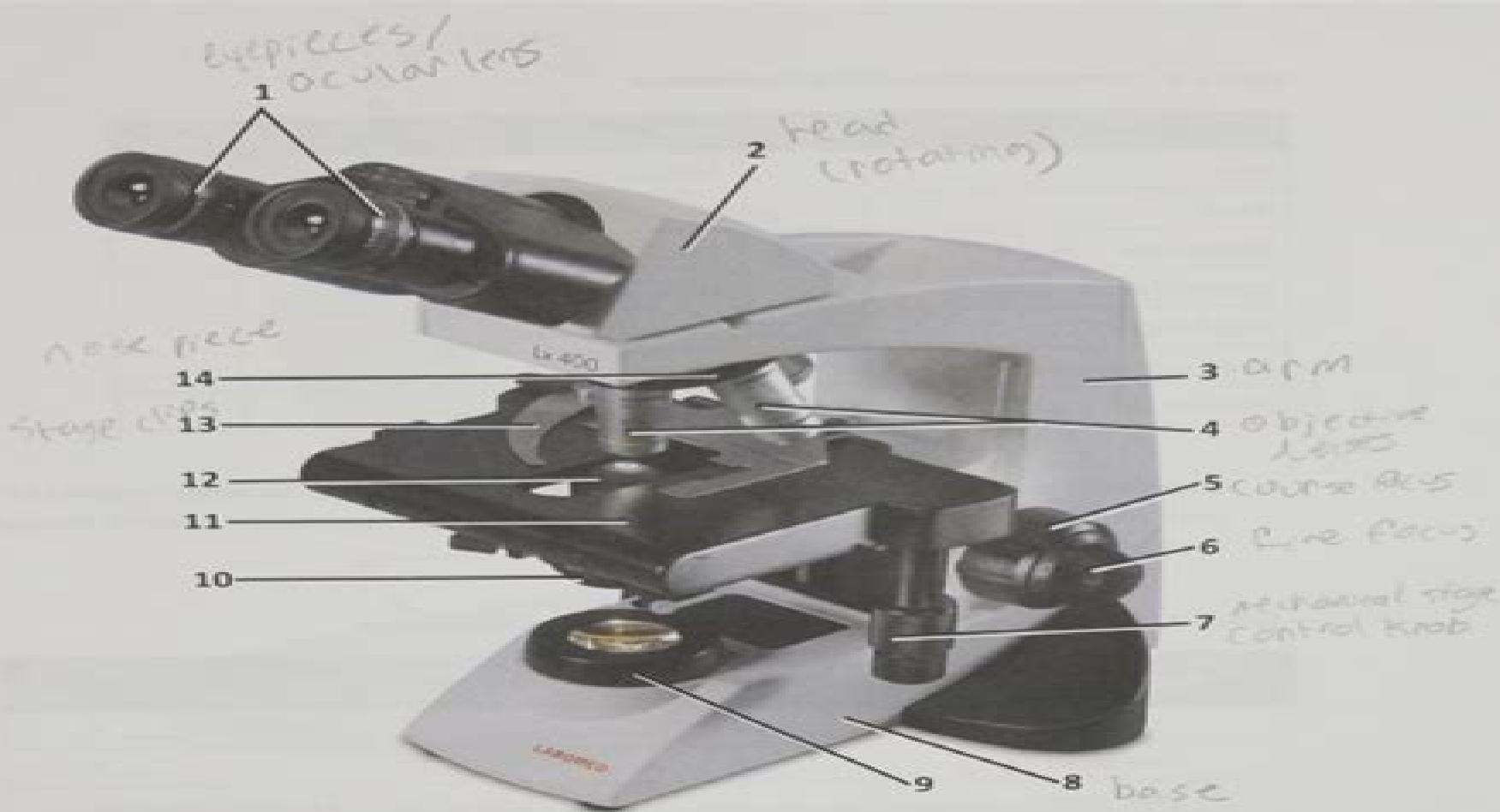
Figure 3. 1. Parts of the compound light microscope (Photo courtesy of Labo America, Inc.)
