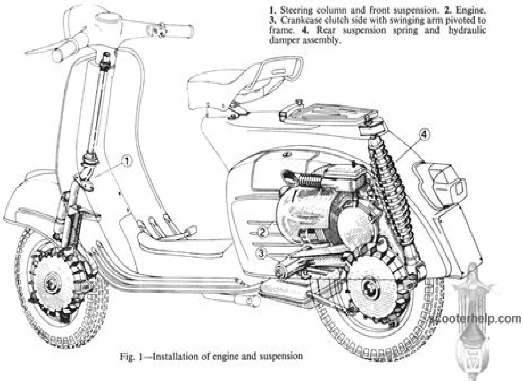
Fig. 1—Installation of engine and suspension
