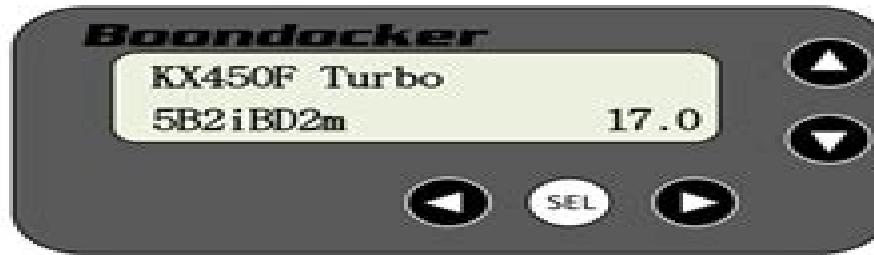
There are five buttons used to navigate through the Boondocker Control box.
