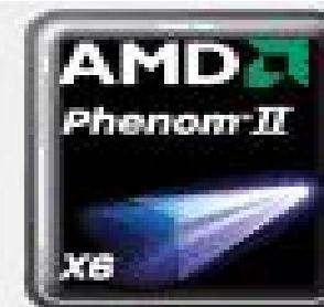
**Specification** **AMD Phenom(tm) II X6 1090T Processor**Family **F** Model **A** Stepping **0**Ext. Family **10** Ext. Model **A** Revision Instructions **MMX(+), 3DNow!(+), SSE (1, 2, 3, 4A), x86-64, AMD-V****Clocks (Core #0)**Core Speed **4200.4 MHz**Multiplier **x 12.5**Bus Speed **336.0 MHz**HT Link **2688.2 MHz****Cache**L1 Data **6 x 64 KBytes** 2-wayL1 Inst. **6 x 64 KBytes** 2-wayLevel 2 **6 x 512 KBytes** 16-wayLevel 3 **6 MBytes** 48-way
