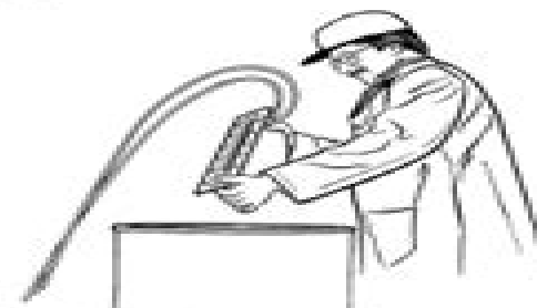
Install a plug in the air vent valve and put a cap on one of the aftercooler water hose tube. Attach regulated air pressure to the other water hose tube. Pressurize the core to 206 kPa (2 bar) (30 PSI) and submerge the aftercooler in water. Inspect for any air leaks. If there leaks or damage, the aftercooler must be replaced.
