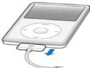
*If your Dock connector is larger than the one shown, squeeze both sides of the connector while removing.*
