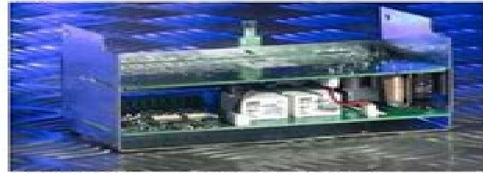
XPC DI6R4: 6 x digital input, 4 x relay outputs
