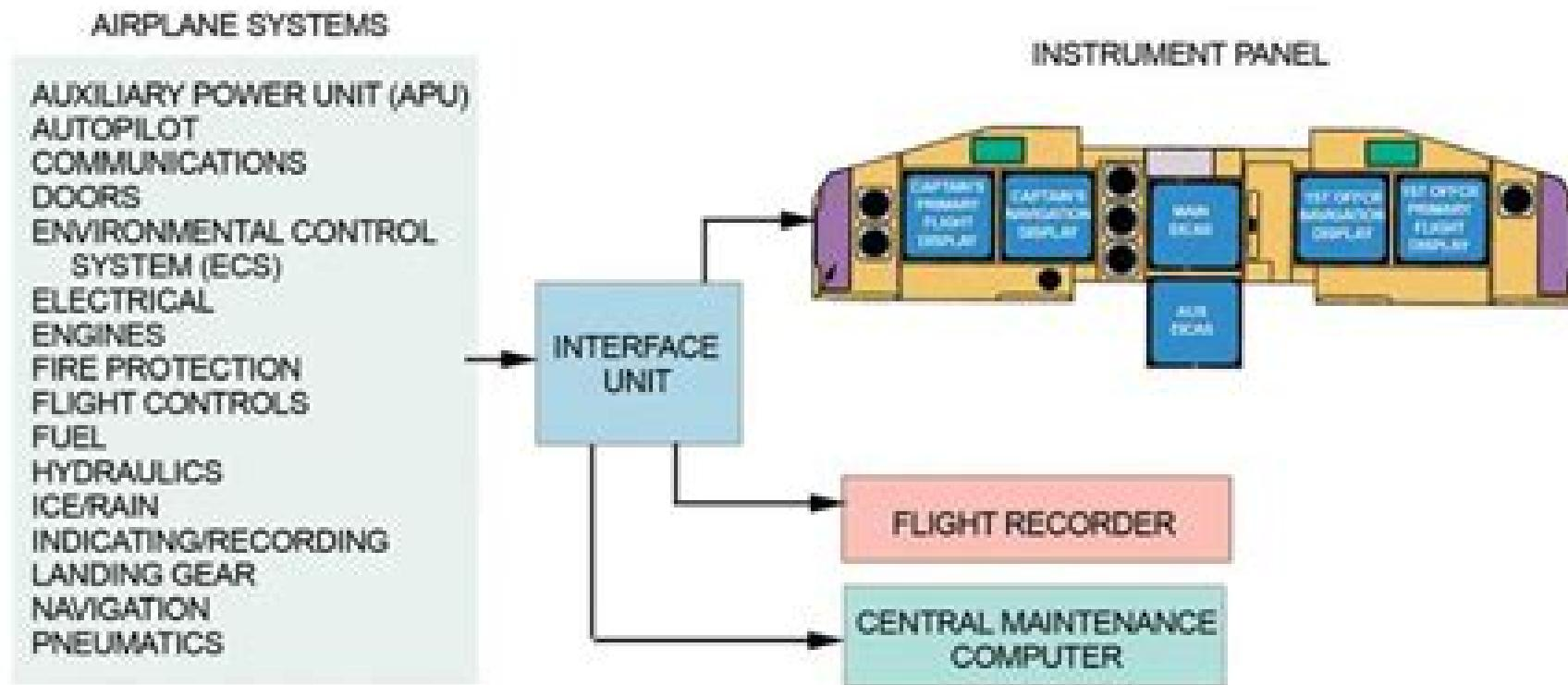
The Boeing EFIS integration with aircraft systems, Flight Recorder and Central Maintenance Computer
