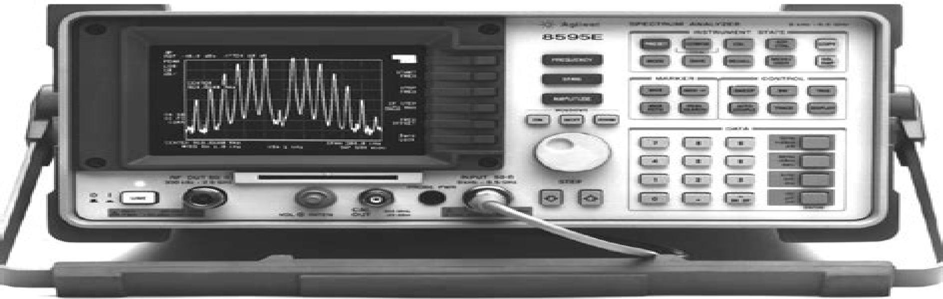
**8591C** Cable TV Analyzer (1 MHz to 1.8 GHz)
