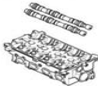
4. Install the cam carrier assembly.
