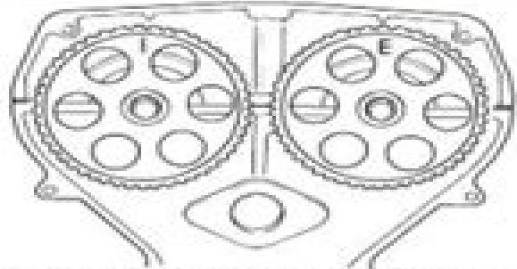
3. Install the camshaft after lubricating the journal of camshaft with engine oil.
