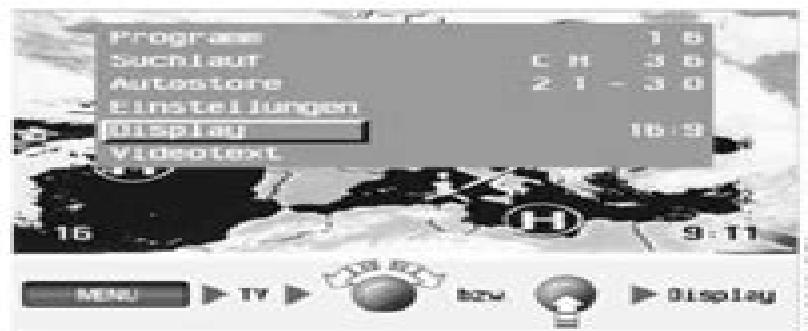
1. Turn or press the right rotary button. The TV menu is displayed on the screen.
