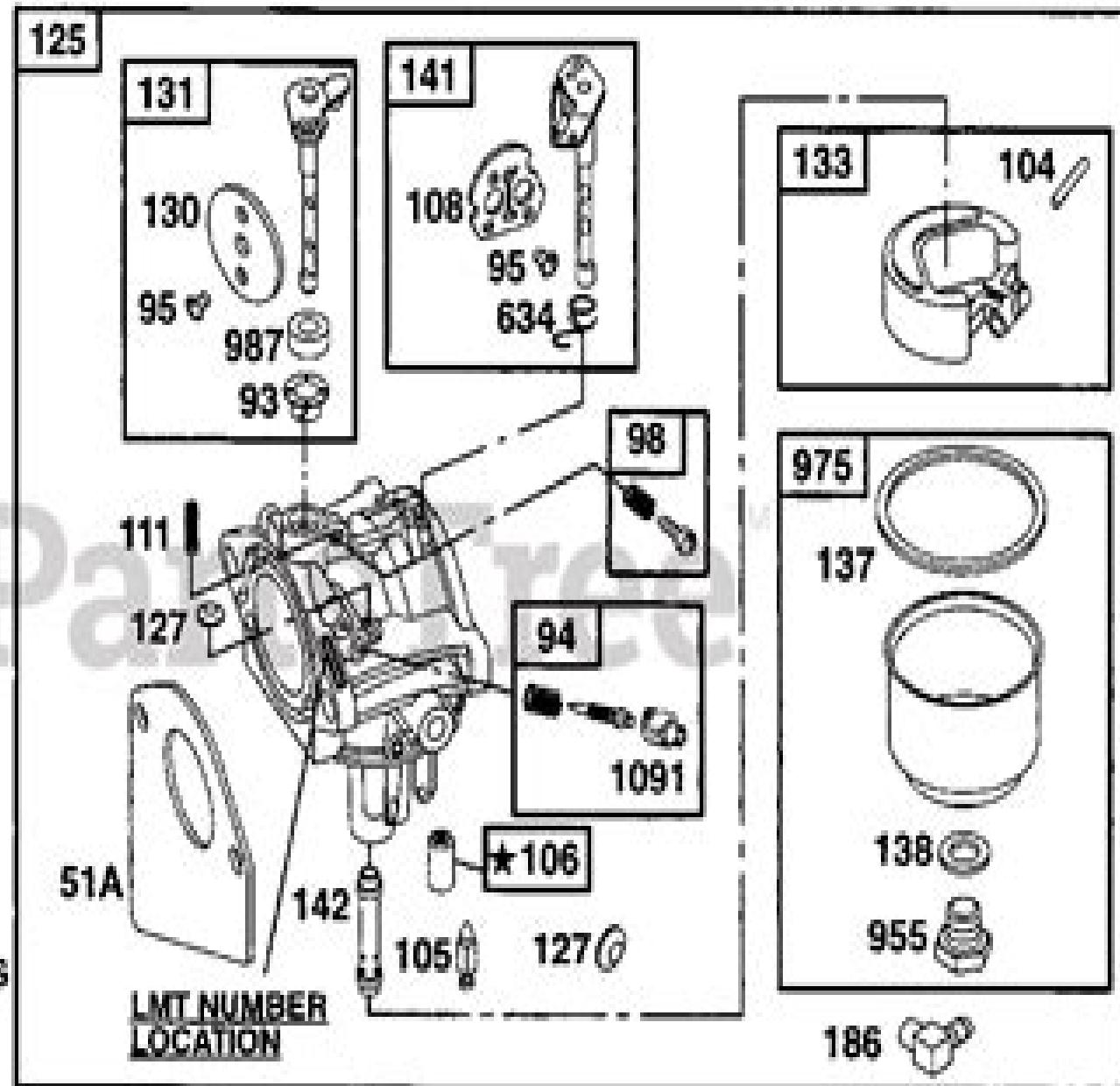
THIS CARBURETOR SERVICES BOTH CHOKE-A-MATIC AND MANUAL CHOKE SYSTEMS
