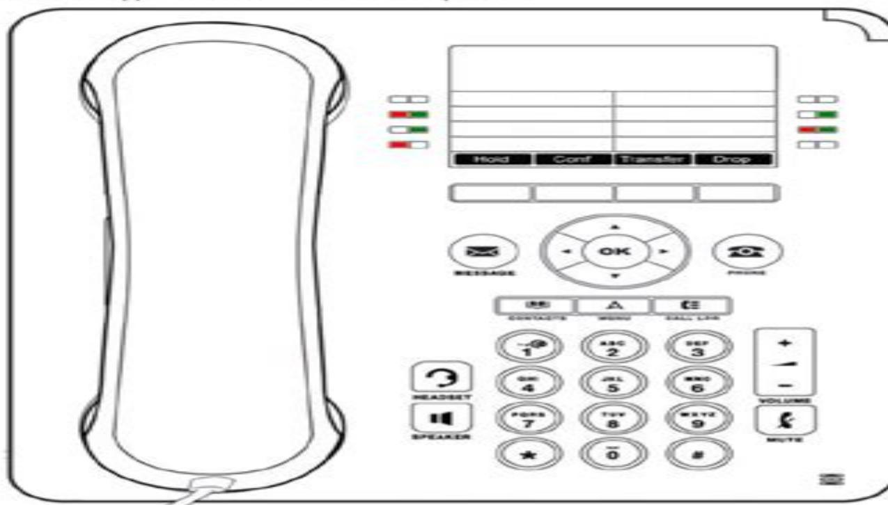
The phone supports 24 programmable call appearance/feature buttons. The labels for these are displayed in the main display and can be controlled by the adjacent buttons.
