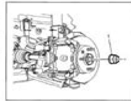
6. Insert the right wheel drive shaft (1) and tighten to 250 Nm (224 lb ft).
