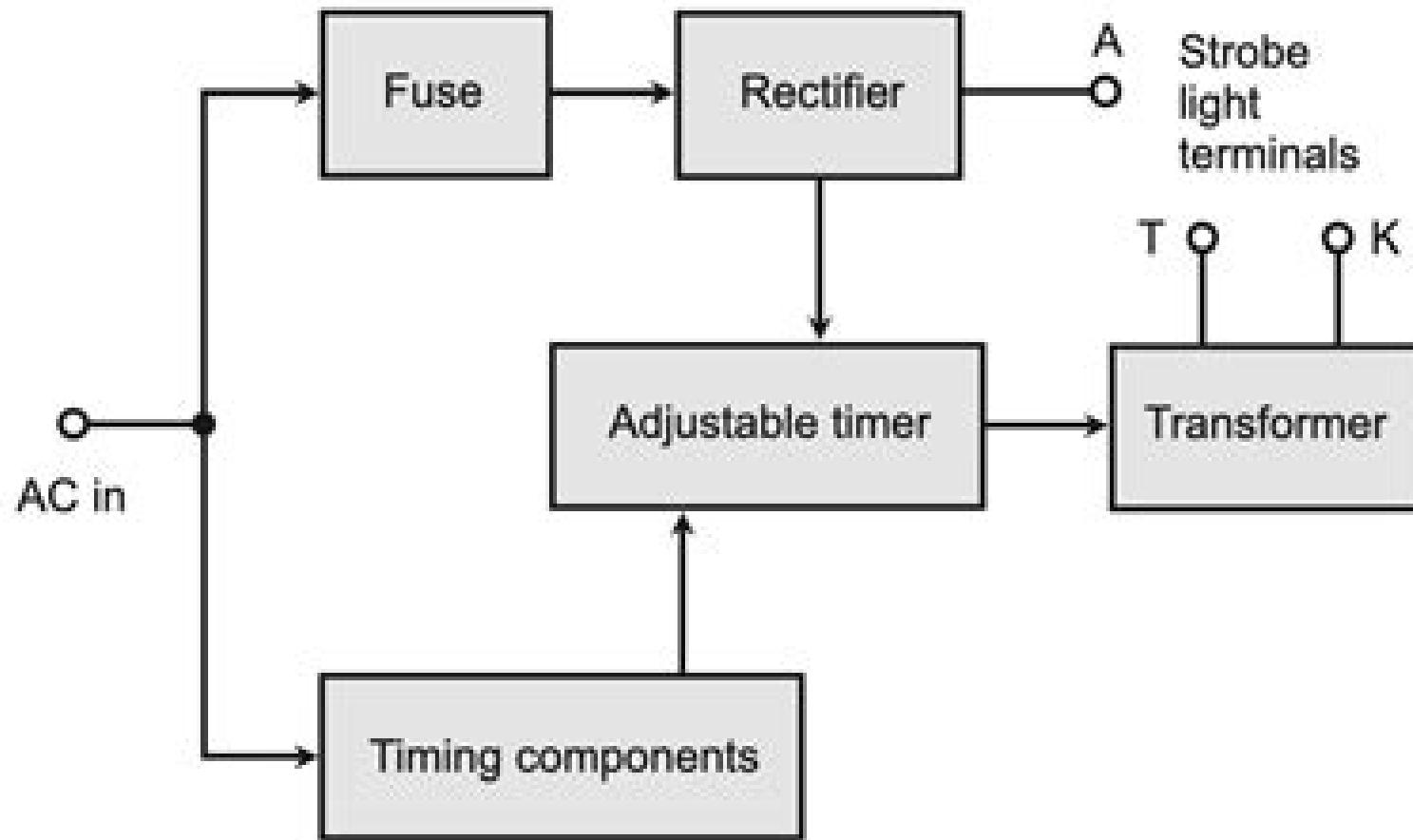
A circuit providing power to a strobe light
