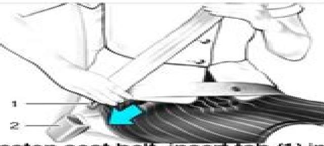
To fasten seat belt, insert tab (1) into buckle (2). Press the red button on buckle to release. Seat belts must be fastened until parking position is reached and vehicle is at full stop.
