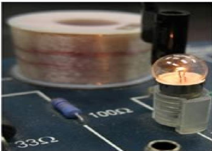
This lit bulb is part of an AC circuit. The coil of wire in the background would have no effect on a DC circuit, but is a key component of an AC circuit. It is called an "inductor."
