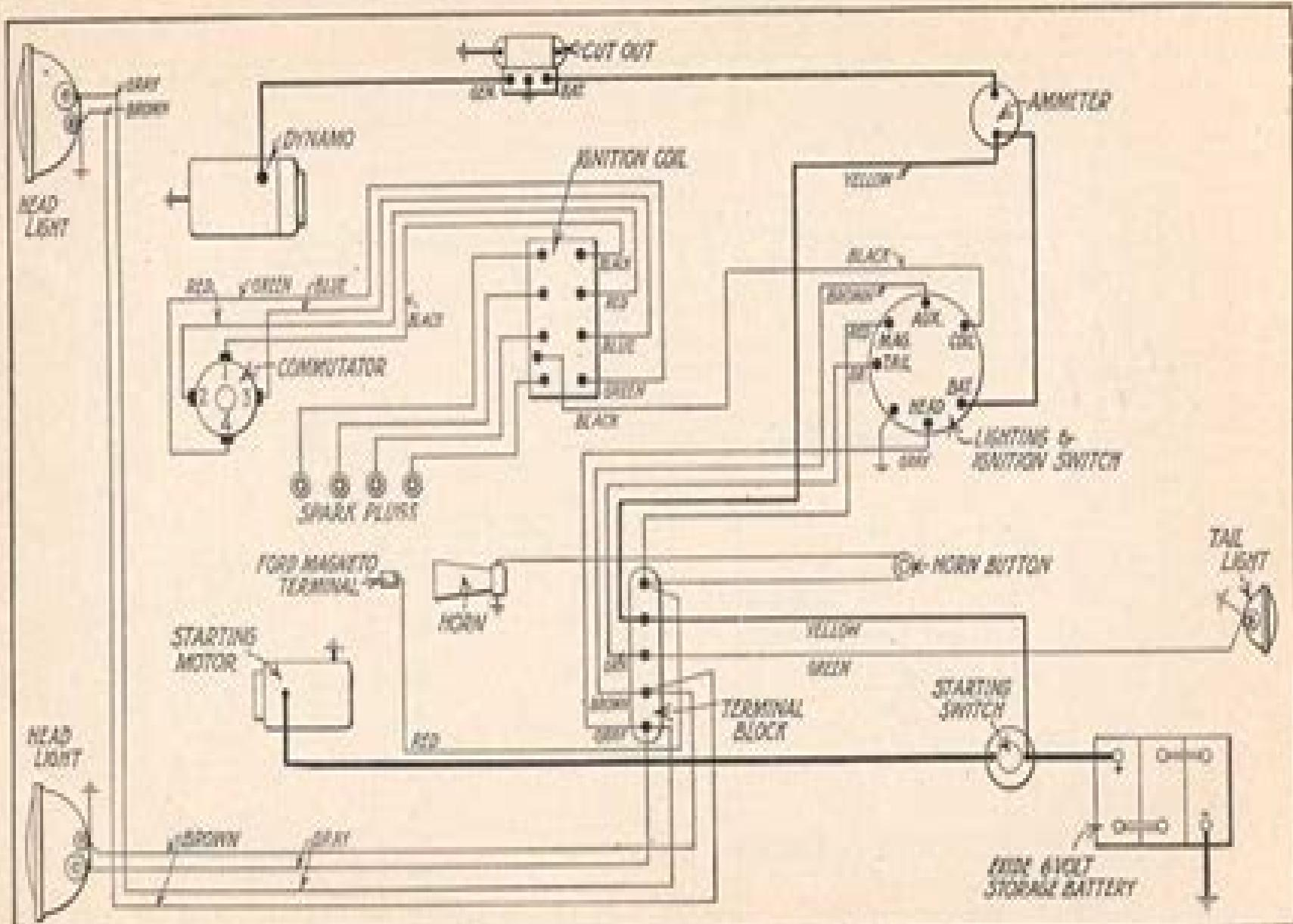
Fig. 17. Wiring Diagram with Cutouts on Dash
