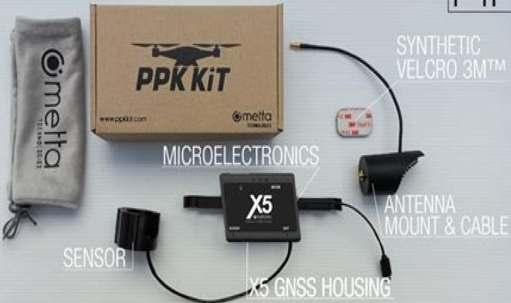
Image: X5 PPK Module Components.
