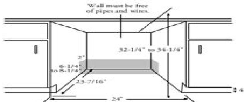
Electrical and water supply should enter through the shaded area and come up through the right side of the machine. Maximum of 4" from the back wall and 8" from the floor. There cannot be any electrical connections in this area.
