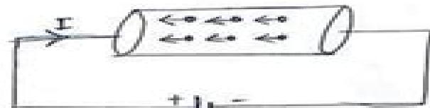
(Current due to flow of charge in a conductor)
