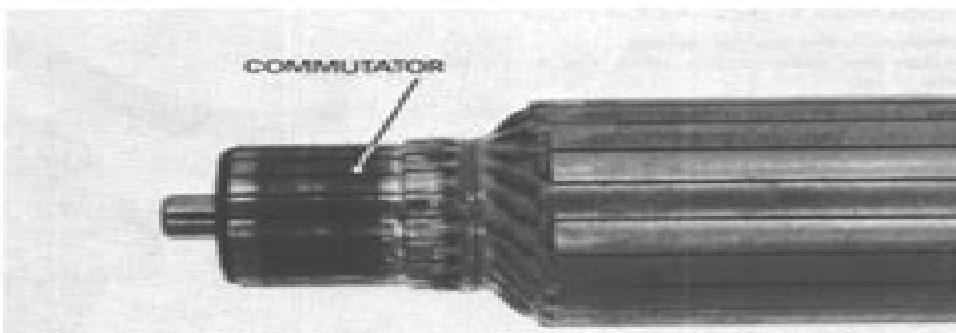
Check for continuity between pairs of commutator bars, and also between commutator bars and armature shaft.
