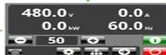
Press Apply Load to start the load test.
